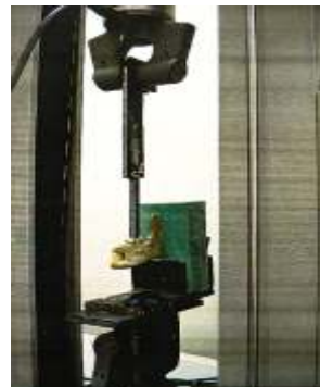
Fig 4 : Testing the strength with Instron machine
